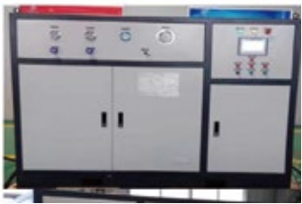
The "Large-Diameter Steel Pipe Burst System" was independently developed for the steel pipe bursting industry.
